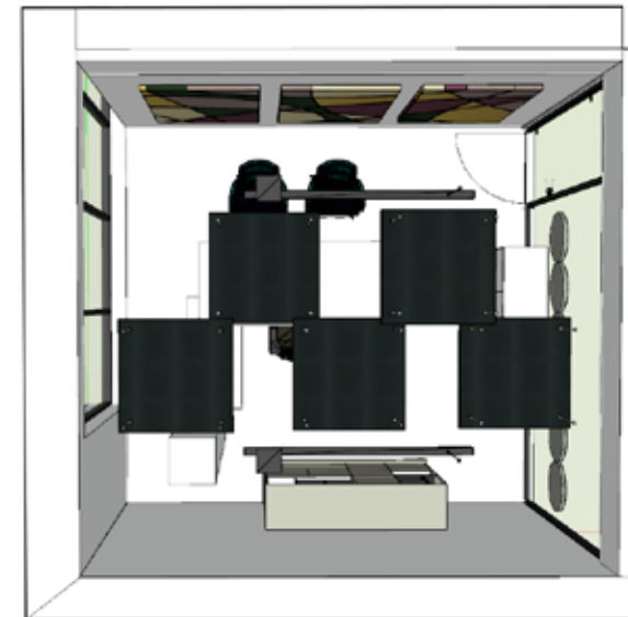
Room after acoustic adaptation - top view
